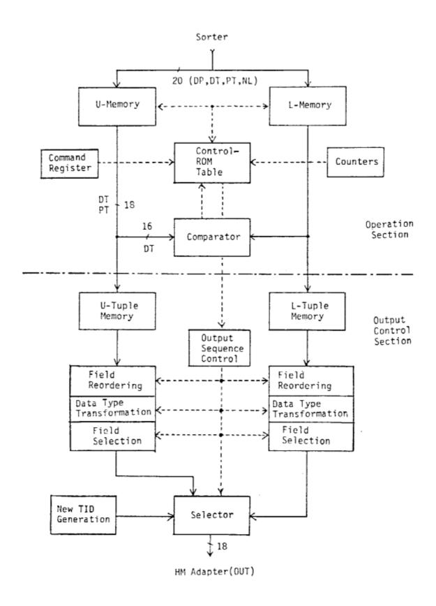
Fig. 5 Block diagram of the merger
