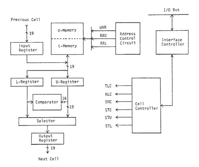
Fig. 4 Block diagram of sorting cell
