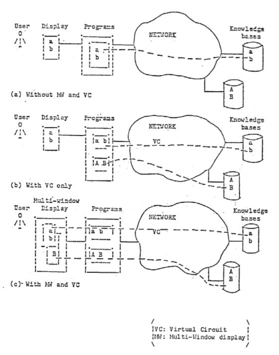
Fig. 3-1 Visualization of Network Environment
