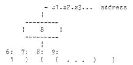
The appropriate cell is located by the memory controller scanning the delimited string structure from the left.
