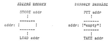
PUT may only store into an "empty" memory cell and TAKE may only remove a non-empty contents, replacing it with "empty". Poth operation may be viewed as polling a memory cell until the cell is in the correct state. (Note STORE and LOAD operations are unaffected by the "empty".)
